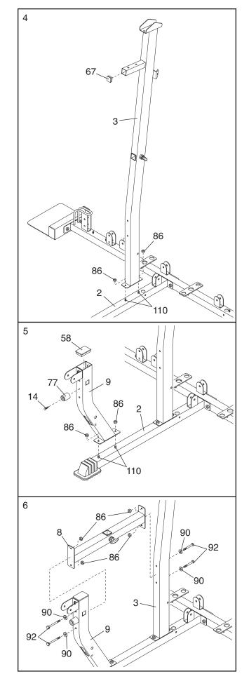
Press a 2" x 3" Inner Cap (58) into the top of the Squat Upright (4). Slide the Squat Upright onto the two indicated 5/16" x 2 1/2" Carriage Bolts (110) in the Long Base (120). Finger tighten a 5/16" Nylon Locknut (86) onto each Carriage Bolt. Do not tighten the Nylon Locknuts yet.
